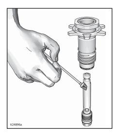
8. Grease o-ring and place on outside diameter ring groove.
