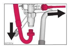
5. Slide pump out of the drive houshing.
