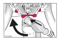
2. Turn pump retaining nut to free pump rod cover.
