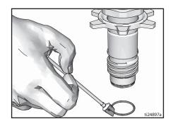
Clean seat thoroughly. Reassemble intake valve with a seat, ball, and new o-ring. Seat may be flipped over and used on other side.
