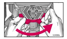
Use a hammer to turn pump retaining nut an additional 1/8 to 1/6th turn or 45° to 60°.
