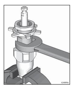
11. Install o-ring onto packing nut. Torque to 75 ± 5 ft-lb (101.7 ± 6.8 N•m) or additional 1/2 turn from hand tight.
