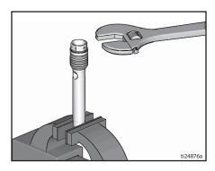
Clean and inspect parts. (The piston has a special thread locking/sealing patch. Apply thread sealant to the threads.
